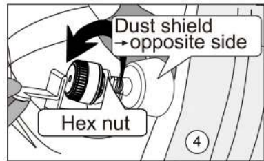
D) Tighten hex nut in an anti-clockwise direction.
