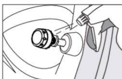
5. Check air leakage by spraying soapy water
