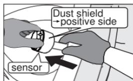
6. Place the dust shield on the hex nut and sensor.
