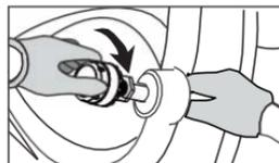
3. Screw the sensor onto the valve
