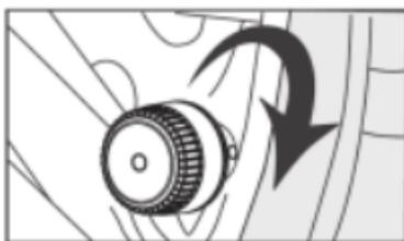
The monitor beeps and stores the tyre position with that sensor ID. If it does not register within a few seconds, unscrew the sensor and try again.
